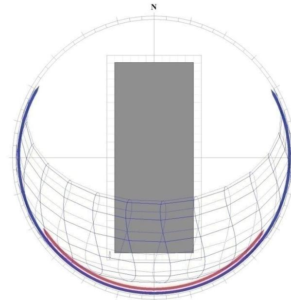
The top building orientation uses 6-8% less energy in Des Moines than the bottom due to less heat gain in the summer and more in the winter.
