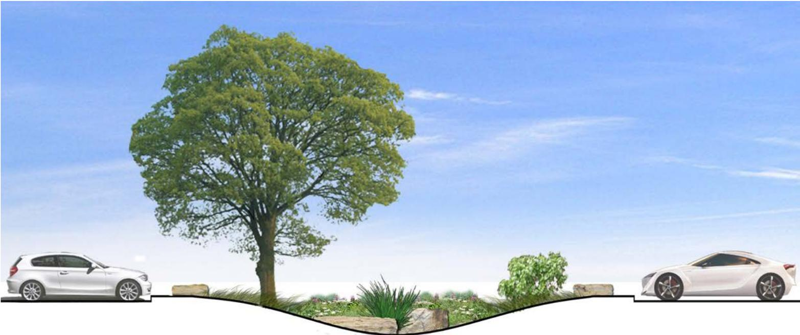
Stormwater runoff from parking lots and other impervious surfaces should be filtered through bioswales, left, or other infiltration methods first before draining to a storm water line.
